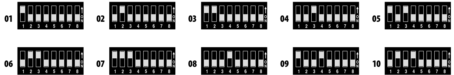
Fig. 7: Address DIP Switch Settings
