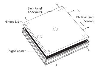
2. Place the back panel on the wall surface using a level to make sure it's straight. Use a pencil to mark the locations of the mounting holes on your wall surface. Drill your wall surface. The diameter of the four (4) corner mounting knockouts is 1/4" and the conduit knockout is 7/8".
