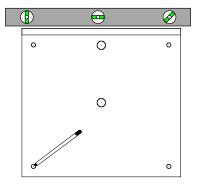
**3.** Pull your electrical through the back panel and attach the back to the wall surface using appropriate fasteners.
