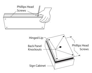
2. Place the back panel on the wall surface using a level to make sure it's straight. Use a pencil to mark the locations of the mounting holes on your wall surface. Drill your wall surface. The diameter of the (4) four corner mounting knockouts is 1/4" and the conduit knockout is 7/8".
