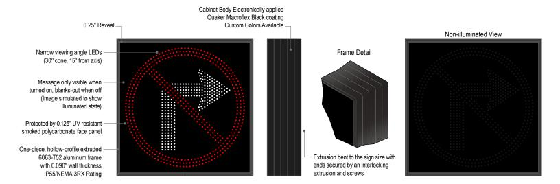
Outdoor/indoor blank-out signs with an IP55/NEMA 3RX cabinet, narrow angle LEDs and contrasting black face The sign message is formed by visible LEDs that illuminate when activated and blank-out when deactivated
