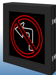
DOT Series NO LEFT TURN R3-2 Cabinet 24"h × 24"w × 5"d Viewable window 18" × 18"w
