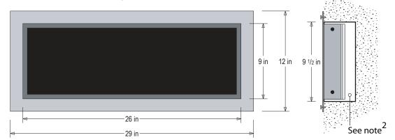
Note<sup>2</sup>: Allow clearance behind sign per local code or per electrical fittings.
